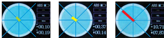
within the tolerance (green) slightly out of the tolerance (yellow) seriously out of the tolerance (red)
