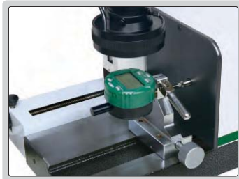
check digital indicators (detect digits on screen)
