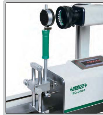
check bore gages
